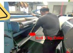
Furthermore, the employer did not shut down the operation of the machine while cleaning the dirt on the roller curtain on the passive roller, which caused the victim to be caught by the roller in the cooling section of the molding machine and died after receiving medical treatment.
