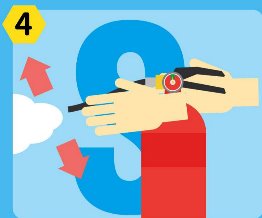
Spray the foam from the fire extinguisher left and right at the base of the fire
